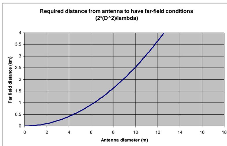
All calculations in this text are based upon the assumption of far-field antenna patterns of the FSS receive antenna. It can be seen that the required distance to be in the far-field ranges from some few hundred metres for small antennas to some few kilometres for large antennas. If the distance between the IMT-Advanced station and the FSS receive antenna is smaller than this, the assumed far-field antenna pattern may not give correct calculated interference levels.
